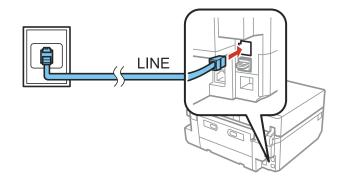
**Note:** If you have a DSL or ISDN connection, you must connect the appropriate DSL filter, or ISDN terminal adapter or router to the wall jack to be able to use the line for faxing or voice calls using your product. Contact your DSL or ISDN provider for the necessary equipment.
